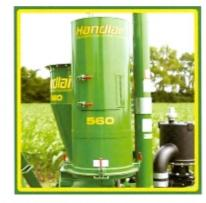
360° swivel discharge cyclone for loading from side, corner, or rear.
