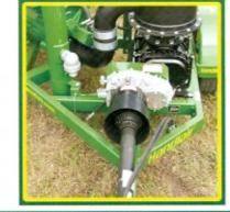
Direct smooth power transmission is provided by the gearbox drive. eliminating side load to the blower.
