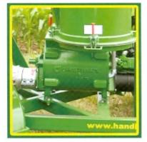
The blow-through airlock is self-cleaning with adjustable tips and endplates for increased performance and longevity. The remote hydraulic airlock valve provides forward / off / reverse airlock control.
