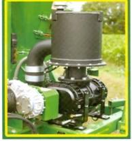
The high pressure positive displacement blower and patented silencer provide increased vacuum capabilities and quiet operation.
