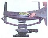
Place vacuum box on the airlock and slide locking hooks around the rear airlock flange.
